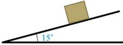
$$F_{gx} = F_g \sin \theta = 4 \times 10 \times \sin 15^\circ = 10.4 \text{ N}$$
