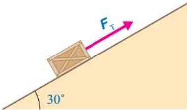
$$F_{gx} = F_g \sin \theta = 20 \times 10 \times \sin 30^\circ = 100 \text{ N}$$
